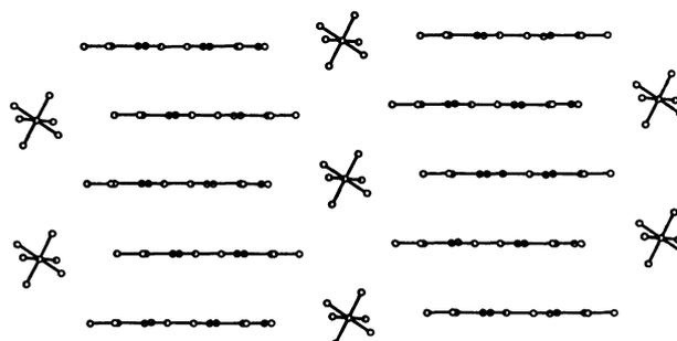
Fig. 1. — Side view of the TMTSF stacks.
