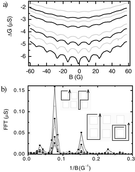
FIG. 1. (a) Conductance versus magnetic field between 25 and 220 mK. (b) Fourier transform of the MC (after subtraction of the envelope) for different temperatures. Left (right) inset: Some orbits contributing to the first (second) harmonic.
