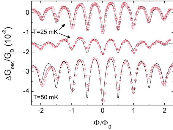
FIG. 4 (color online). Comparison between experiment (symbols) and theory (continuous line) for the oscillating part of the conductance for sample A ( $\square$ ) ( $G_D = 3.7 \times 10^{-5}$  S), sample B ( $\star$ ) ( $G_D = 5 \times 10^{-6}$  S) with  $V_g = -0.15$  V corresponding to  $W = 240$  nm and  $l_e = 170$  nm, and sample C ( $\circ$ ) ( $G_D = 2.6 \times 10^{-5}$  S) (shifted down for visibility). The only adjustable parameter is the amplitude of the oscillations.
