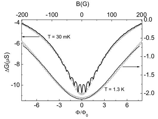
FIG. 3. High field MC, the continuous lines are the experimental data, and the dots are the fits with Eq. (4). Parameters of the fits are  $l_e$  and  $W$  at 30 mK, and  $L_\phi$  and  $l_e$  at 1.3 K.
