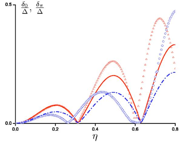
FIG. 2. Gaps at  $\chi=0$  (circles) and  $\chi=\pi$  (triangles) as a function of the spin polarization  $\eta$  in a short junction with  $k_F d=10$ . Equations (13) and (14) provide a good approximation for small  $\eta < 0.1$  (dash-dotted line,  $\delta_0$ ; solid line,  $\delta_\pi$ ).
