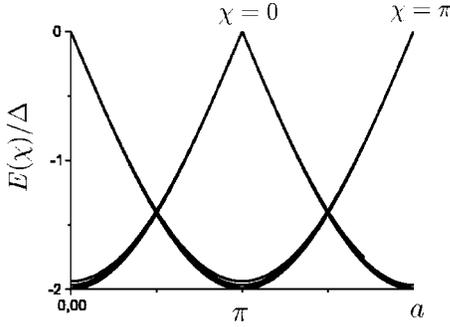
FIG. 7. Zero-state energy  $E(\chi=0, a)$  and  $\pi$ -state energy  $E(\chi=\pi, a)$  for  $\eta=0.1, 0.3, 0.5$ . The intersections of the different curves remain in the vicinity of  $a=\pi/2$  and  $a=3\pi/2$ .
