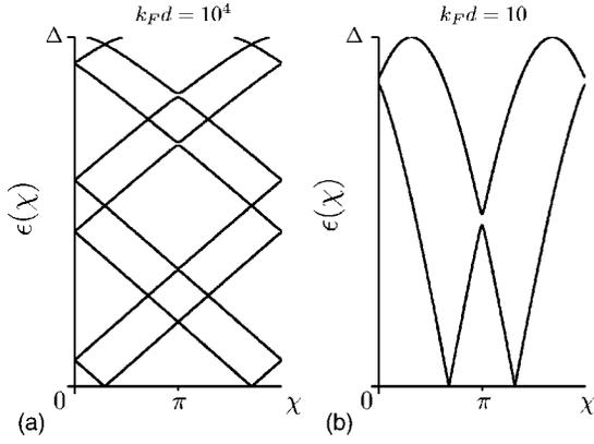
FIG. 1. Spectrum of a clean SFS junction in the perturbative limit  $\eta=0.1$  and for  $\Delta/E_F=10^{-3}$ . Two examples are shown: (a) long junction with  $k_F d=10^4$  ( $d=5\xi_0$ ) and (b) short junction with  $k_F d=10$  ( $d=0.05\xi_0$ ). Gaps open for  $\chi=0$  and  $\chi=\pi$  due to the presence of ordinary reflection. There are two zero energy Andreev levels located at the phase differences  $\pi \pm \Delta k_{\epsilon=0, \eta} d$ .
