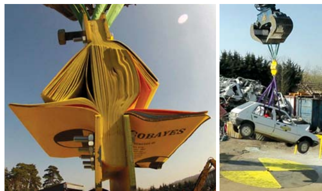
FIGURE 1. THE FRICTION FORCE generated by the two interleaved phone books on the left is enough to support a car, as illustrated in the scene at right from the show On n'est pas que des cobayes! , aired in France on 2 May 2014. (© France 5/2P2L, used with permission.)
