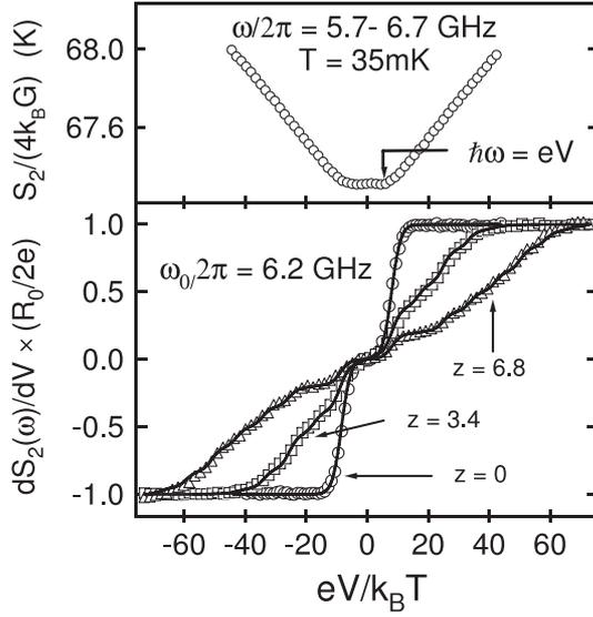
**Figure 2.** Top: measured noise temperature  $T_N = S_2(\omega)/(4k_B G)$  of the sample plus the amplifier with no ac excitation. Bottom: measured differential noise spectral density  $dS_2(\omega)/dV$  for various levels of excitation  $z = e\delta V/(\hbar\omega_0)$ .  $z \neq 0$  corresponds to photo-assisted noise. Solid lines are fits with equation (10).
