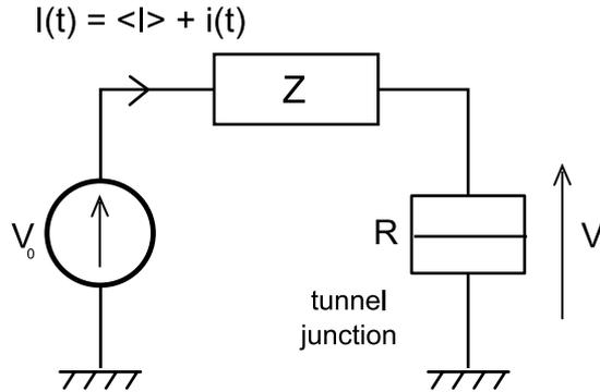
**Figure 1.** Schematics of the experimental setup. The tunnel junction is connected in series with a voltage source (voltage  $V_0$ ) through a given impedance  $Z$ . Current fluctuations  $i(t) = I(t) - \langle I \rangle$  are measured using an ammeter with a bandwidth  $\Delta f$  while the voltage  $V$  across the tunnel junction can be measured using a voltmeter.
